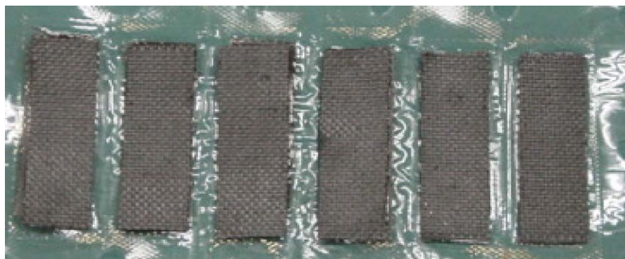
Fig. 1. A monopolar membrane–electrode assembly consisting of six pairs of electrodes.
